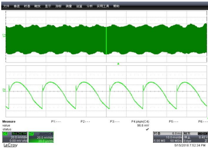
Figure 16: 90Vac/60Hz 5V/3A \Delta V=96\text{mV}
