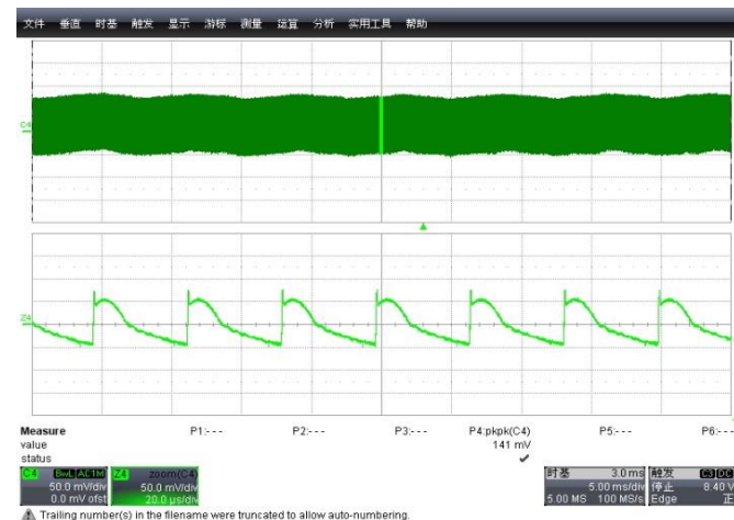
Figure 31: 264Vac / 60Hz 20V/2.25A \Delta V=141\text{mV}
