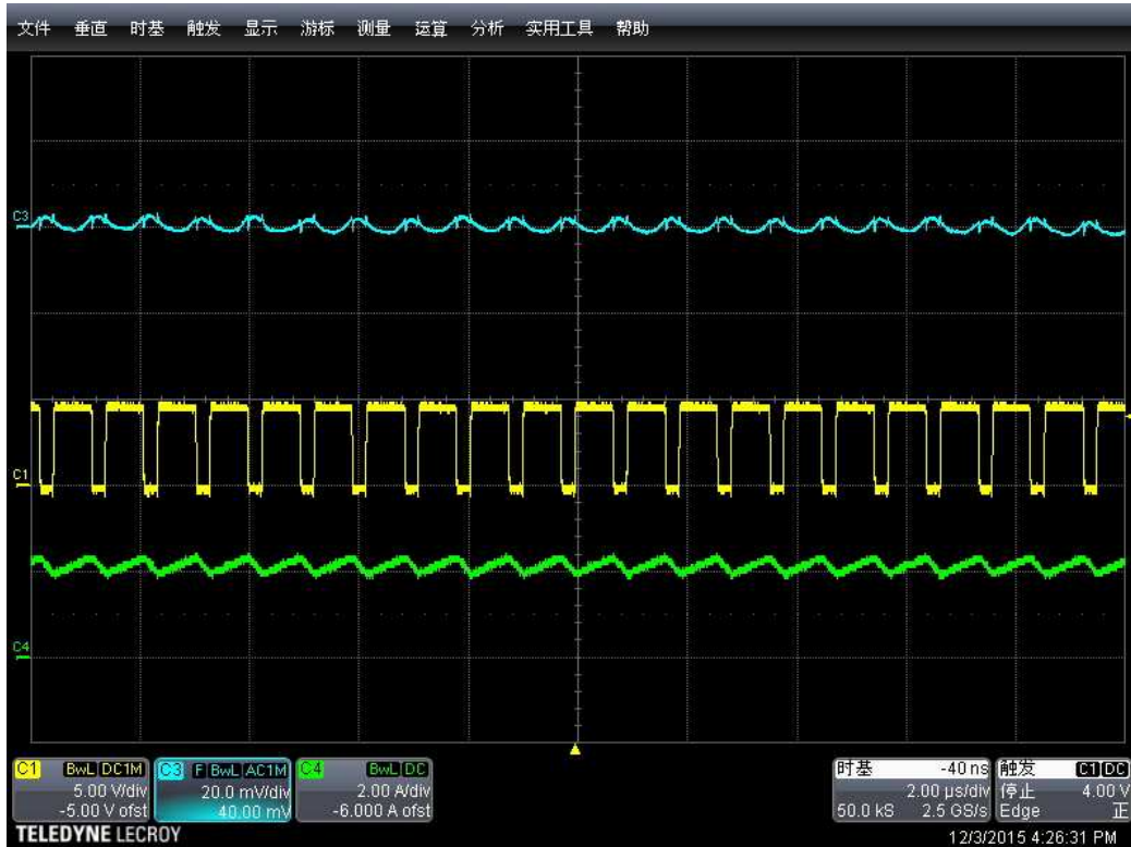
Operation waveform at I_{out}=2A (Blue-VoutAC; Yellow-Vsw; Green-IL)
