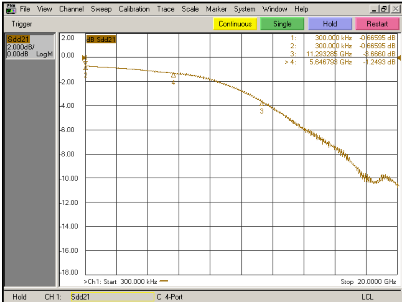
Figure-4, the -1.2493db /5.646Ghz (11.2Gbps) differential insertion loss of PI3BDS12412A (reference for PI3BDS12212A)
