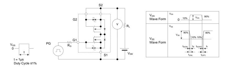
Test Circuit 8  $t_{D(ON)},\,t_{R},\,t_{D(OFF)},\,t_{F}$
