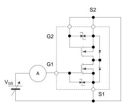
Test Circuit 2 I<sub>GSS</sub> When FET1 is measured, between GATE and SOURCE of FET2 are shorted.
