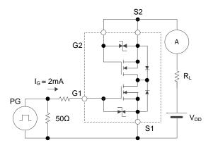
Test Circuit 9 Q<sub>G</sub>
