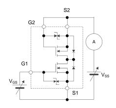
$\begin{array}{c} \text{Test Circuit 4} \mid Y_{\text{fs}} \\ \Delta I_{\text{S}} / \Delta V_{\text{GS}} \end{array}$
