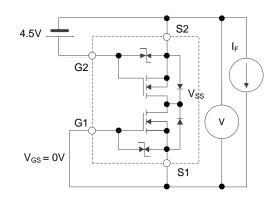
$\label{eq:FET} \begin{array}{l} \mbox{Test Circuit 6 $V_{F(S-S)}$} \\ \mbox{When FET1 is measured, FET2 is added $V_{GS}$ +4.5V.} \end{array}$
