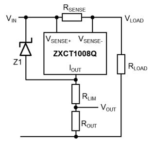
Figure 1. ZXCT1008Q with Additional Current Limiting Resistor  $R_{\text{LIM}}$  and Zener Z1
