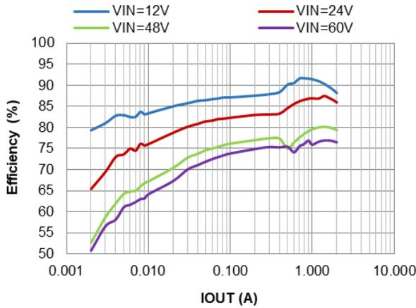
**Figure 9. PFM Efficiency vs. IOU, VOUT=3.3V, L=8.2µH**
