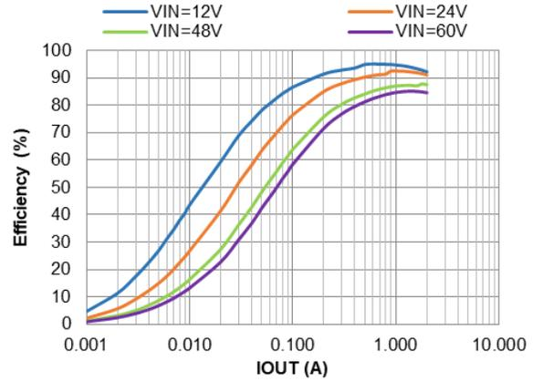
**Figure 8. PWM Efficiency vs. IOU, VOUT=5V, L=10µH**
