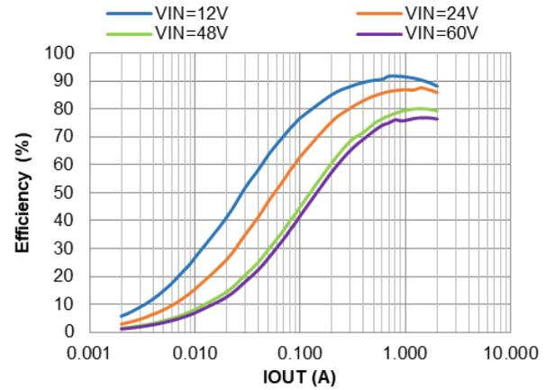
**Figure 10. PWM Efficiency vs. IOU, VOUT=3.3V, L=8.2µH**
