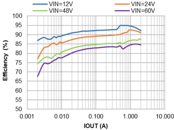
**Figure 7. PFM Efficiency vs. IOU, VOUT=5V, L=10µH**
