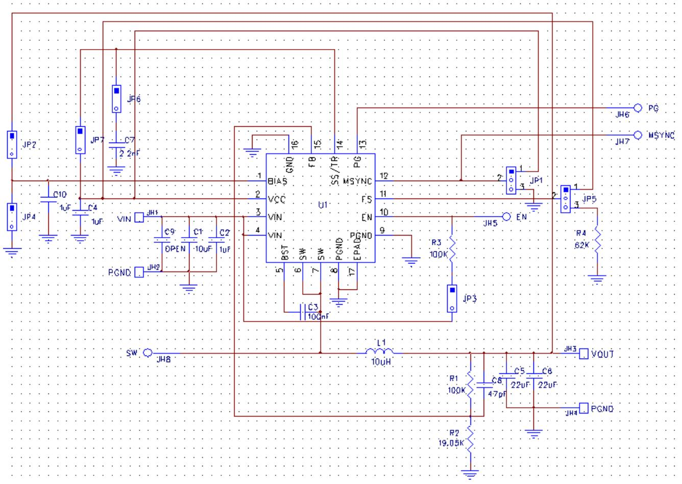
Figure 2. AP66200QFVBW-EVM Schematic
