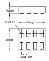
The X2-DFN1210-8 is one of the world's smallest 8 pin packages used for logic.
