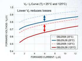
V<sub>F</sub> measured per diode
