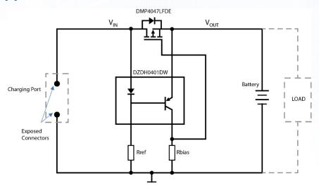
$V_{IN}$  >  $V_{OUT}$  minimizes forward losses.  $V_{IN}$  <  $V_{OUT}$  high isolation, blocks battery discharge path protecting charging port.
