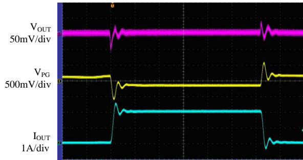
Load Transient ( V_{CTRL}=V_{EN}=5V , V_{IN}=2.2V , I_{OUT}=0 to 2A )
