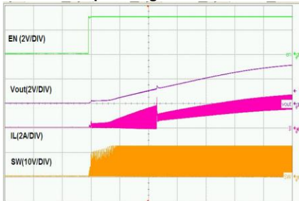
Startup Through Enable 2A
