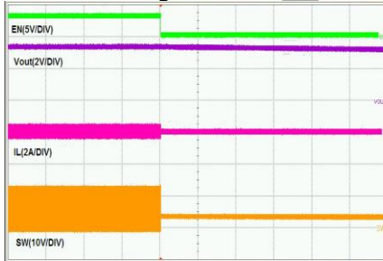
Shutdown Through Enable_no load
