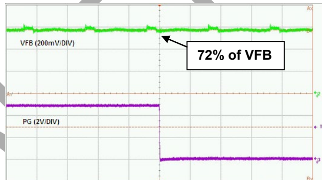
Time- 1 \mu s /div Powergood Falling Threshold
