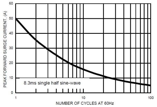
FIG.2- MAXIMUM NON-REPETITIVE SURGE CURRENT
